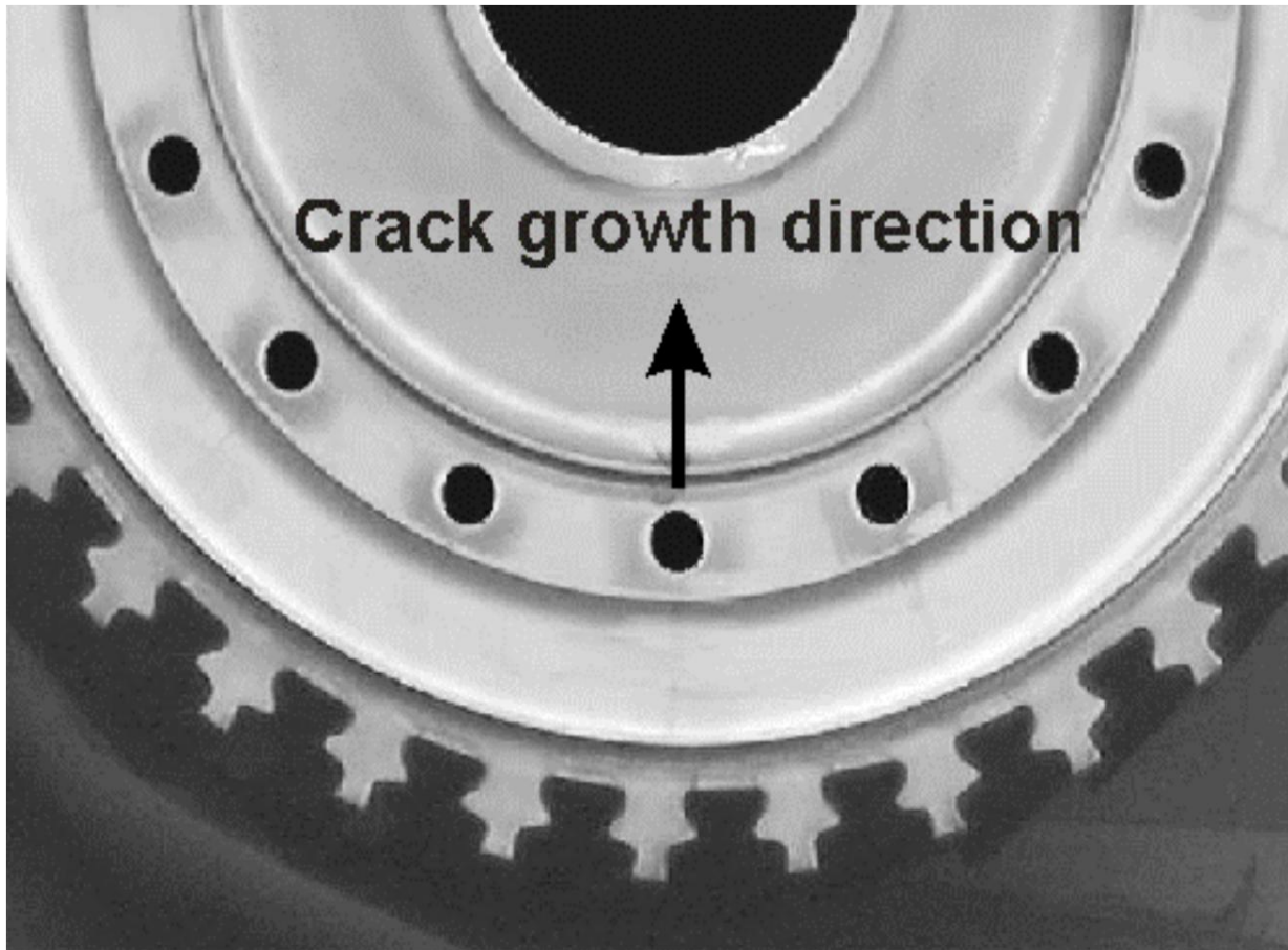
Disc geometry and crack growth direction
