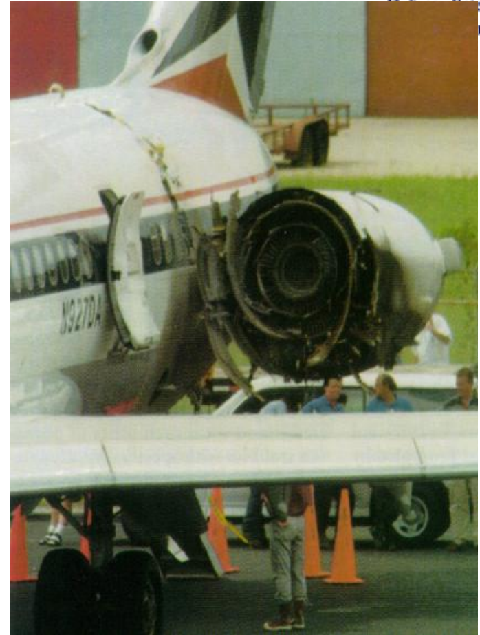
JT8D engine uncontained failure on a MD-88 in 1996
