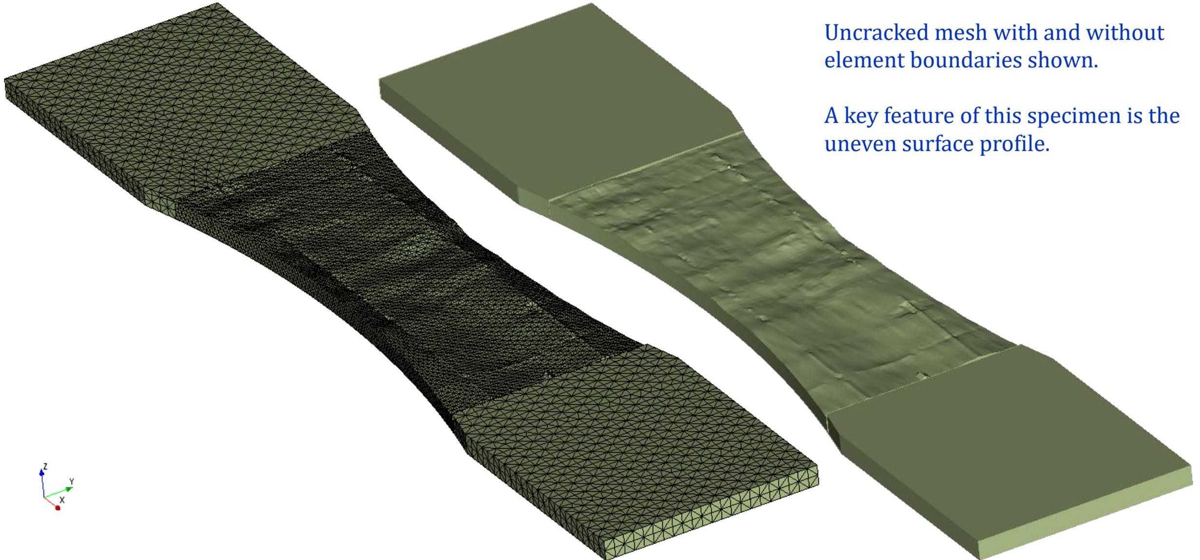
Uncracked mesh with and without element boundaries shown.
