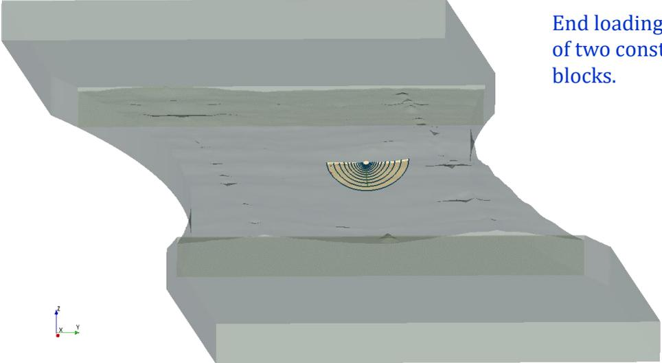
End loading is a sequence of two constant amplitude blocks.
