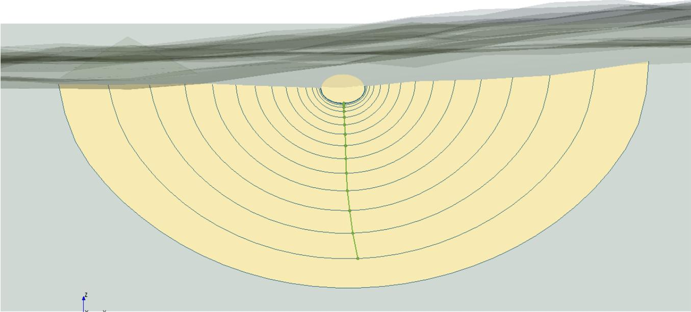
Green line is trace of middle point of the crack front used for xy plots (next slide)
