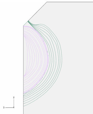
Figure 13: Predicted growth of 'IGA' crack under cyclic load
