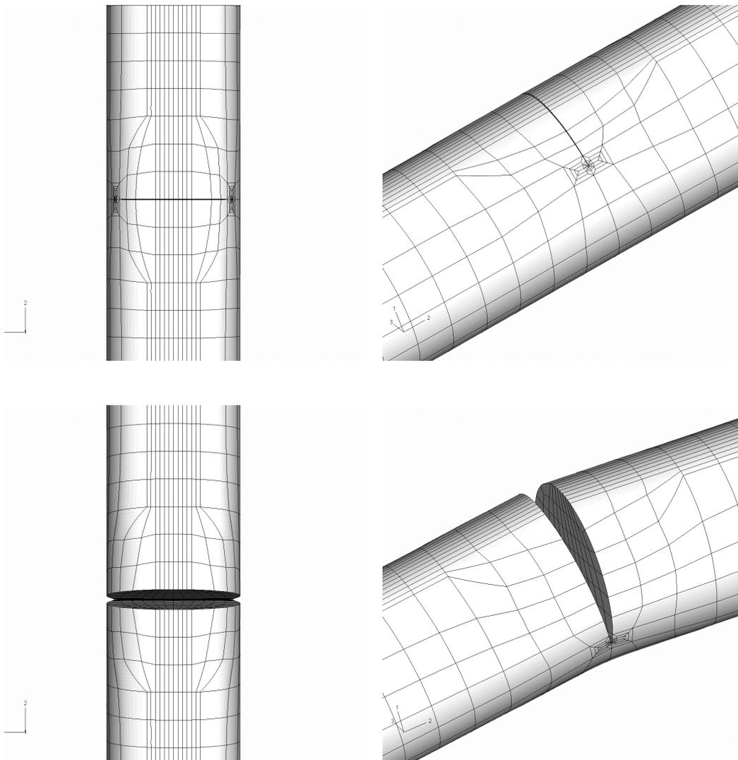
**Figure 3: Two stages during the analysis for tension-only loading (deformations magnified).**
