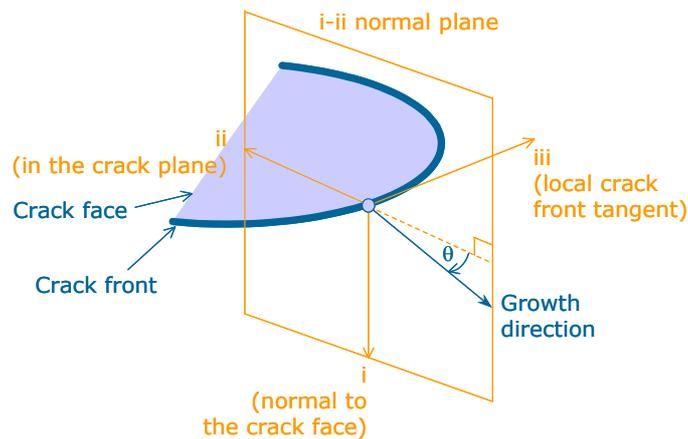
**Figure 1: Local out-of-plane crack growth for a point on a 3D crack front.**
