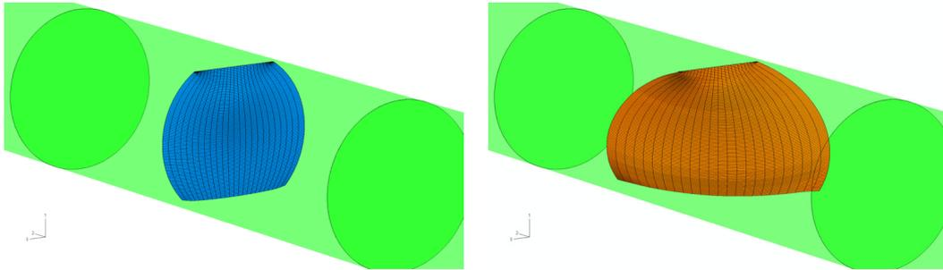
**Figure 5: Comparison of tension-only and in-phase tension-torsion crack development.**
