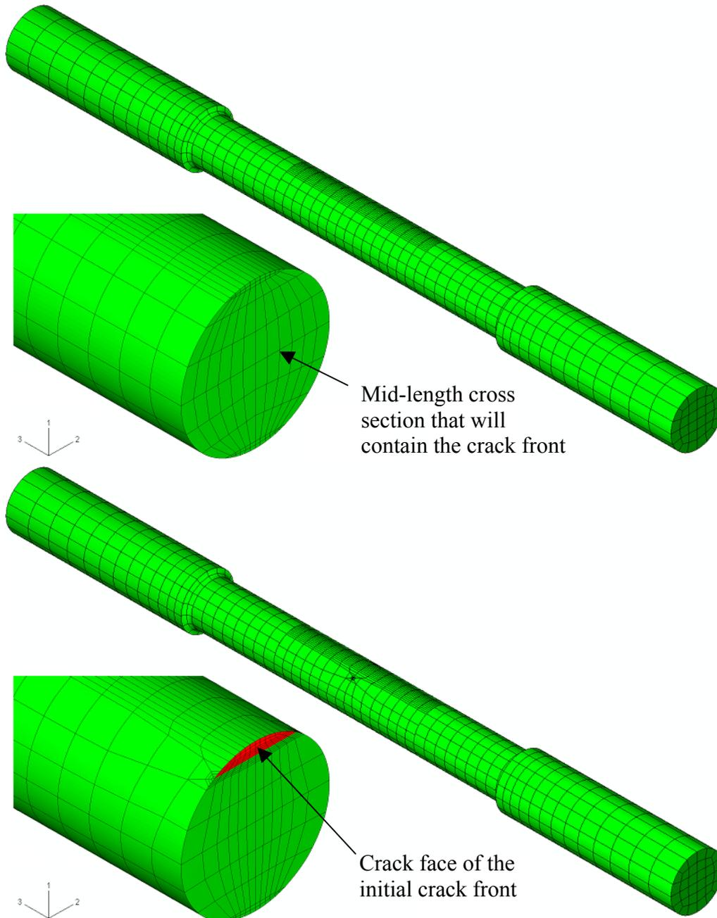
**Figure 2: Uncracked (top) and initial cracked (bottom) meshes for the tension-torsion shaft analyses.**
