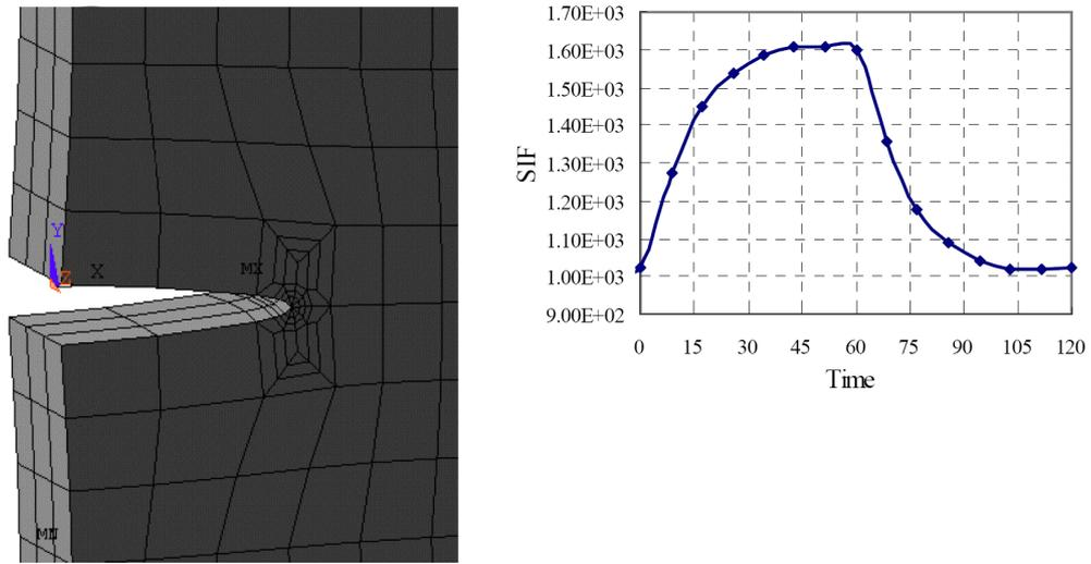
**Figure 9: Stress intensity factor through a thermal cycle with constant applied tension [3].**
