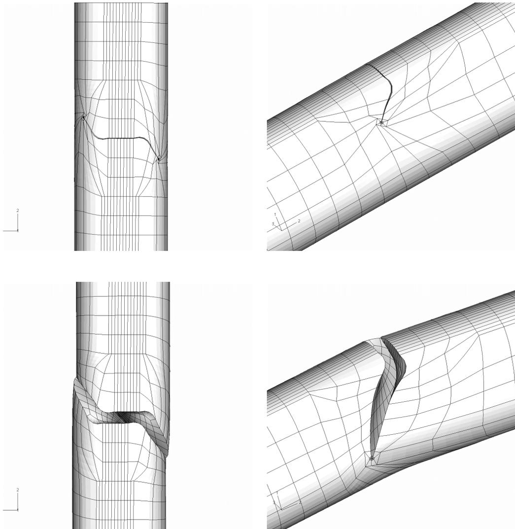
**Figure 4: Two stages during the in-phase tension-torsion loading (deformations magnified).**
