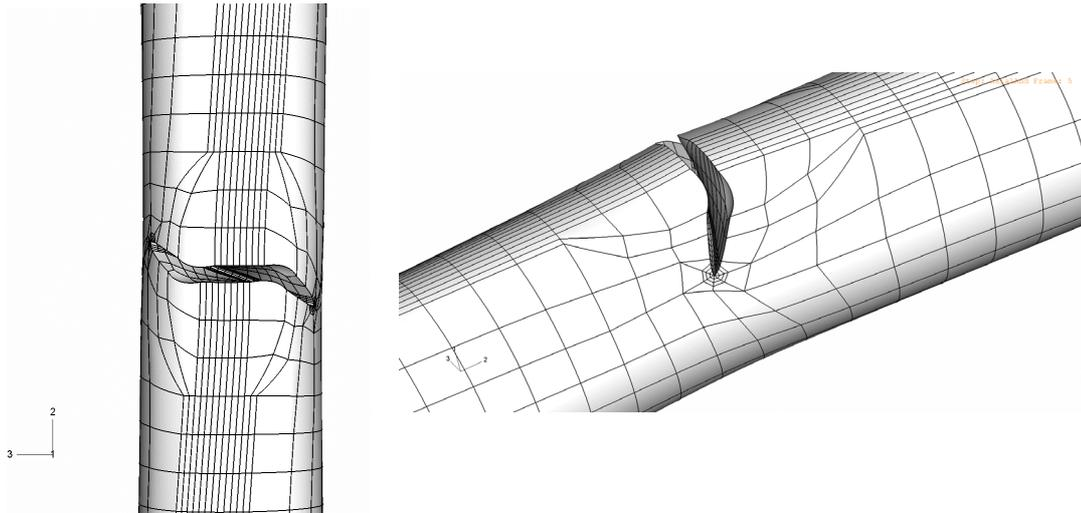
**Figure 7: Stage during the constant tension-cyclic torsion loading (deformations magnified).**
