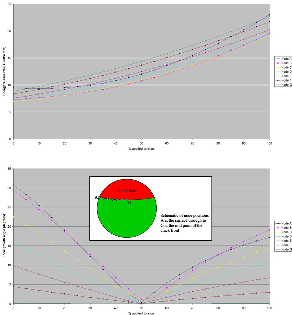
Figure 6: Constant tension and increasing torsion – instantaneous G and out-of-plane angle for nodes along an advanced crack front.
